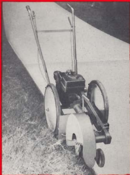
Edging Unit makes quick work of trenching and trimming along drive-ways and sidewalks.
