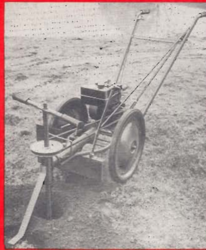
Post Hole Auger digs full 7" holes at rate of one per minute. Designed for safe one man operation.
