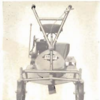
Bicycle type steering with convenient handle mounted throttle control. Front wheels ball bearing mounted. King pins have oilite bronze bushings with ball thrust bearings.
