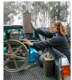
Ellbie (Skatjie) holds the broken, unique exhaust in place on the rare Petter with uncooled head.
