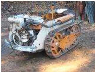
Ransomes MG (market garden) crawler, fitted with Sturmev-Archer engine. This crawler outsold any other make in the UK during its production run.
