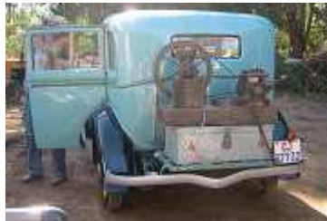
Braams Studebaker called a Rockne. The contraption mounted on the back is a Briggs WMB and small feed mill. The WMB was developed to power domestic washing machines.
