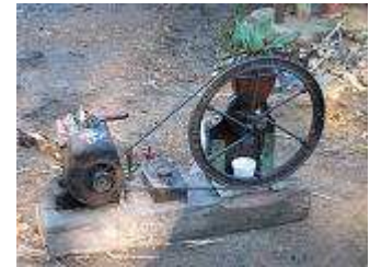
Braams Studebaker called a Rockne. The contraption mounted on the back is a Briggs WMB and small feed mill. The WMB was developed to power domestic washing machines.
