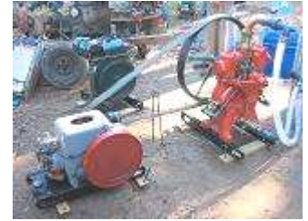
Pompes Fateur pump driven by a 1937 International Harvester LA Petter AP1 behind.
