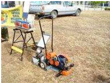
2. My air vane governed 3/4hp Johnson AX468 driving car generator.
