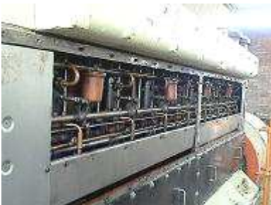
Upper side covers removed for access to the fuel injection pumps. The fuel inlet rail can be seen with curved branches connected to the pumps.
