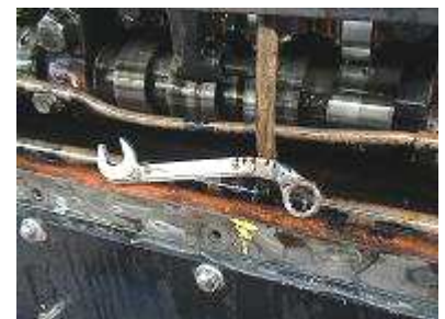
Curved spanner made up for access to the left-hand rear bolt. Even a 'starter spanner' wasn't much help.
