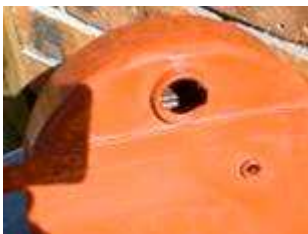
An international LB tank showing the nice shiny tough epoxy coating and light shining through the epoxy where there were rusted holes, the photo taken through the filler cap while holding the tank up to the light.
