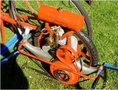
Briggs & Stratton 'motor wheel' that dates from around 1920, it would be interesting to say the least, riding a pushbike with it attached?
