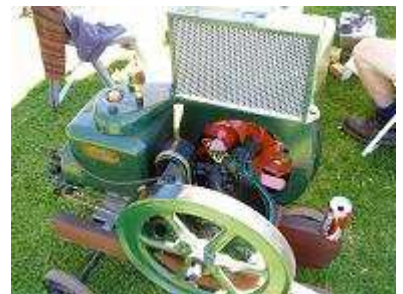
Fairbanks Morse type Z. Note the unusual condenser for boiling water from the hopper.
